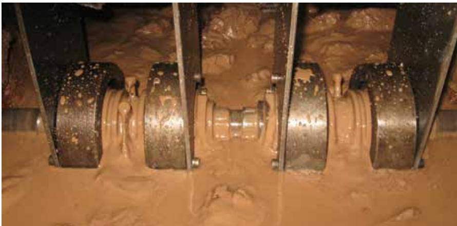
Mudslurry test rig
